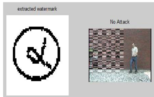
Fig.15. Video watermarked frame without attacks and extracted watermark from watermarked frame
