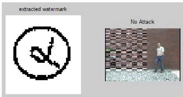
Fig. 9. Video watermarked frame without attacks and extracted watermark from watermarked frame.
